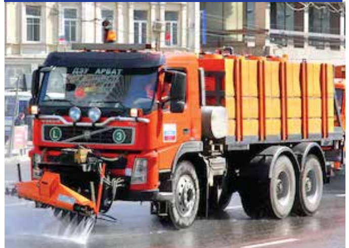
STREET, THUNNEL AND BARRIER WASHING
