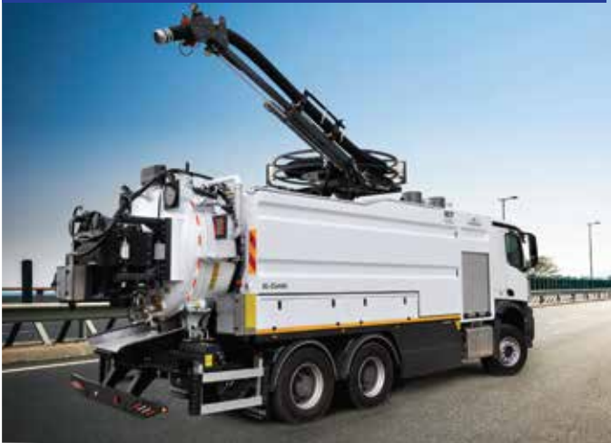
COMBINED SEWER JETTING AND CLEANING
